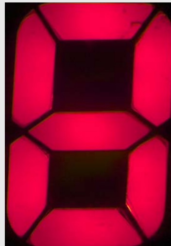
Fig. 2. Hot spot were removed from the 7-segment after optimization of materials and shape.
