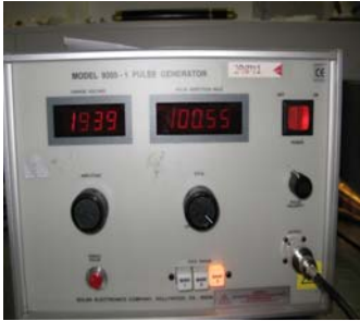
1KV Solar Electronics Company Model 9355-1 trapez generator
