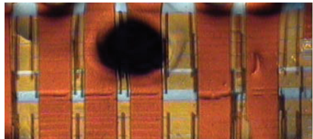
Hot spot analysis - Hot spot detected by use of liquid crystals.
