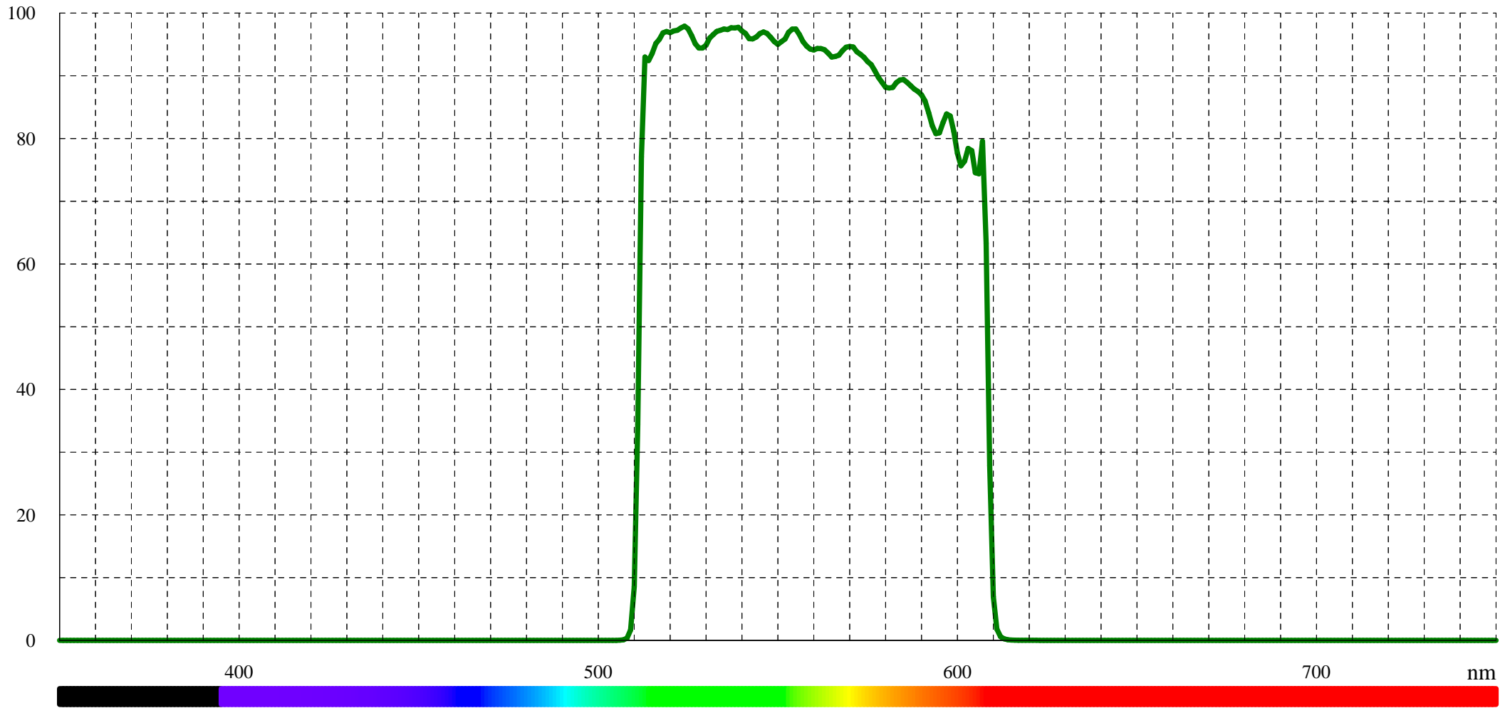
Typical transmission for BP 560/100 (LF101832)
